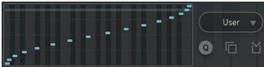
**Q** Button puts the faders to quantized mode for easy pitch assignments.
