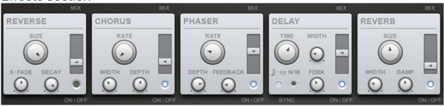
Right beside the Sugar Bytes logo you find the "VIEW" button which switches between Sound- and Effects Section. The effects are running in chain (according to the effects order in the user interface, from left to right) and can be mixed with the original signal.
