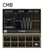
Comb filter that is based on short delay times. This one is good for vowels and resonator sounds.
