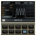
Ripple Filter. A spectral filter that consists of 4 bands that are shifted within the frequency domain.
