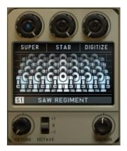
This is a special Super-Saw oscillator thet generates 7 sawtooth waveforms running at a slight pitch offset for a massive sound.
