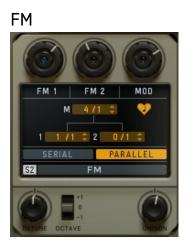
Our idea of easy 3-OP-FM synthesis. A Modulator Oscillator modulates 2 Carrier Oscillators. Two FM algorithms provide a variety of FM sounds that fit snugly to the Cyclop concept.
