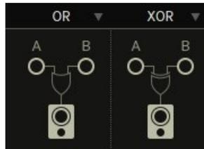
Logic Gates are the key operators of digital computing. They operate with binary values, 0 being LOW (no signal), 1 and above being HIGH (signal). Logic Gates force their inputs follow specific rules, such as: ‘if two triggers happen at the same time, don’t output a trigger’ (NAND). Or, ‘only output a trigger if both inputs happen at the same time’ (AND). For convenience, we’ve included Comparators (>, <, =) which work with all number values (but output a logical 0 or 1).
