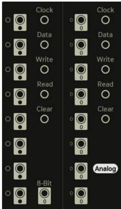
Derived from the classic 4015, the shift register is a data recording device. They allow you store number values within their eight 'memory cells'. What makes the shift register unique is that the cells are arranged in a line, with the output of one cell connected to the input of the next cell. This allows the data from one cell to be 'handed over' to the next cell, until the data is finally discarded (or fed back to the input to cycle continuously).
