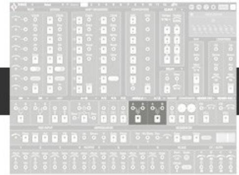
Simple equations for whenever math is needed. This can be for when you need to multiply up the value of the oscillator waveshapes or the envelope signal. Or if you want to subtract 2 octaves (24) from a sample and hold signal.
