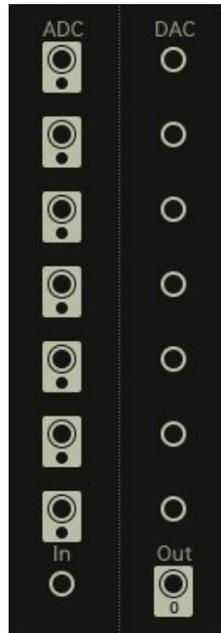
Here we have a 7-bit AD/DA converter. The use of such a converter is to turn analog voltage into digital numbers (bits) and vice versa. A bit is simply a 0 or a 1. In short, the converter will take 'analog' values from 0-127, and spit out a unique combination of seven 0s or 1s (ADC). Or conversely, it will take the sum of seven digital inputs, and output a unique 'analog' value of 0-127 (DAC). This is a perfect range for working with MIDI.
