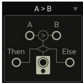
It operates on various conditions, **comparing** inputs  $A$  and  $B$ , and **forwarding** inputs  $C$  (true) or  $D$  (false) to the *output*.
