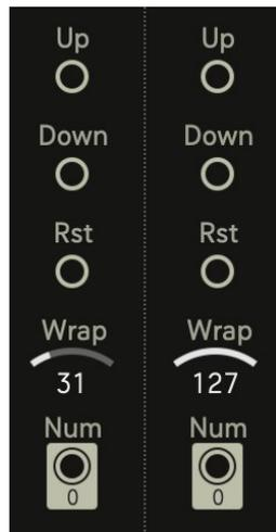
These counters increment values up to, or down from a specified number, set by *Wrap*. A clock/trigger event at the input will tell the counter how much to count by. So, a clock with the value of '1' will tell the counter to count up by ones: 1, 2, 3, 4, 5, 6, etc. And a clock with a value of '2' will tell the counter to count by twos: 2, 4, 6, 8, 10, etc. This occurs until the counter arrives at the *wrap* number, at which point it starts from 0 again.
