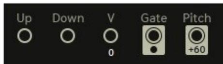
**Up:** Apply triggers to count up through the input voices. Triggers increment according to their number value (count up by 1s or 2s, etc.)
