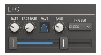
You also can fade in the LFO intensity by using the Fade parameter.
