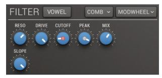
The Modwheel mode works in the same way as the Pitchbend mode, except that it assigns the MIDI modulation wheel to fade between 2 frequencies (or vowels).
