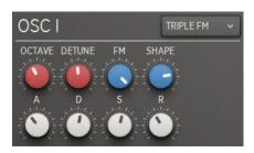
Triple FM is based on frequency modulation of three oscillators. This oscillator provides classic FM sounds, but also unheard-of and inspiring material, from thin and piano-like to fat, detuned and distorted.
