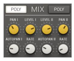
Right between the two oscillators is Unique's Mix section. Here you can adjust level and pan for each oscillator.
