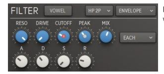
In this mode there is an ADSR envelope, which modulates the cutoff frequency.
