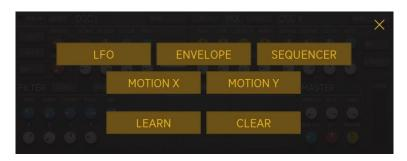
All knobs can be modulated with internal modulators or controlled by MIDI or Host Automation. Just right click on a parameter and a menu with certain modulation sources comes up. The first 5 entries assign a modulator to the knob you just clicked on.
